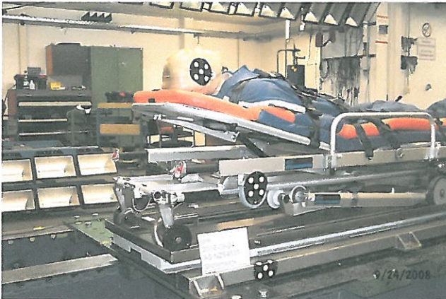
Detail: head end; Tubular brackets for carriage fixation on ambulance tray
