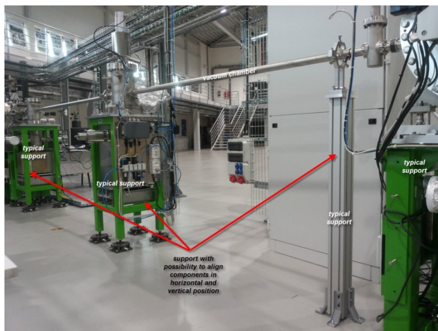
Drawing 4 A model support system of vacuum chamber using metal supports
